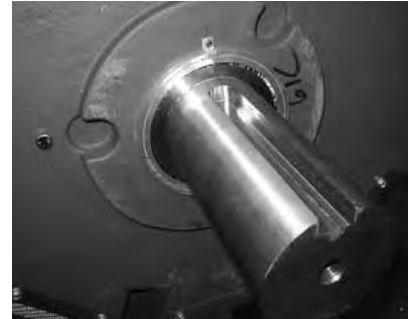
AEGIS® Shaft Grounding Ring Drive End
